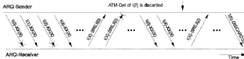
J.A. 15041. In this figure, the transmitter first sends packets 0–3 to the receiver before the receiver sends back its first feedback responses. Due to delay and packet loss, when the transmitter is first notified that the receiver did not receive packet number 2—the second I(X)–SREJ(2) message—the transmitter has already deleted packet 2. The transmitter will then inform the receiver that it can ignore packet number 2 by sending the discard packet message—the I(5)–DISCARD(2) message.
